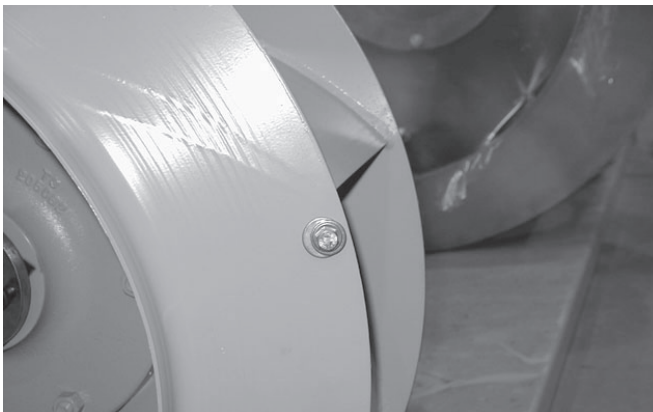
Permanently secured stainless steel bolts, nuts and washers used as balancing weights after paint
