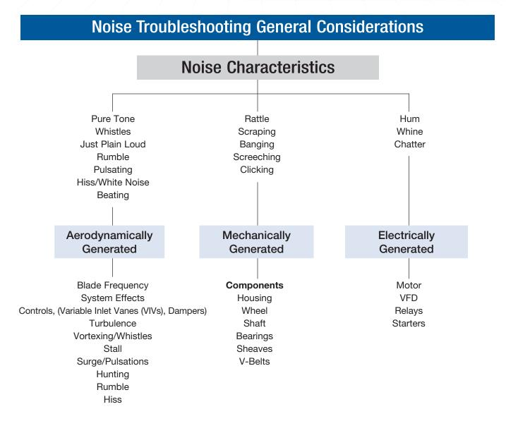
Noise is generally considered low-quality, unwanted sound. The ears sense noise whereas vibration is sensed by touch or feel. Sources of noise can usually be identified by some form of characteristic sound to which we can relate. Words such as tone, rattle, pitch, steady or unsteady, and intermittent are examples. These characteristic words help to define whether the source of the noise is aerodynamic, mechanical, or electrical.
