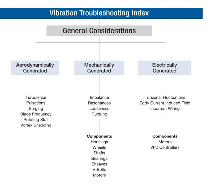
Many different sources can cause vibration. One of the most difficult tasks in troubleshooting fans and systems is the systematic identification of vibration characteristics (amplitude, frequency, location, direction, units of measurement) as a function of operating point location on the fan curve and control settings. Identification of the source can be extremely difficult, in some cases requiring the services of a professional troubleshooter.
