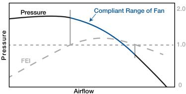
Figure 3: Compliant range of operation of a fan operating at multiple speeds
