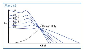
The table below is an example illustrating the fan power savings and the Fan Energy Index (FEI) for various fan sizes all applied at the same design duty point.
