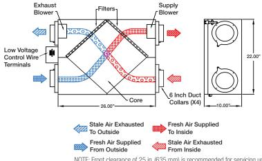
NOTE: Front clearance of 25 in. (635 mm) is recommended for servicing unit. All ducts use 5 in. (125 mm) round collars. MERV 13 upgrade: 485463
