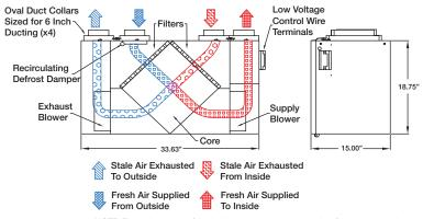
NOTE: Front clearance of 25 in. (635 mm) is recommended for servicing unit. All ducts use 5 in. (125 mm) round collars. MERV 13 upgrade: 485465
