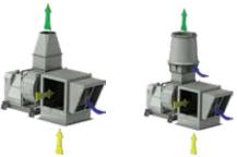
Isolation Damper – Parallel airfoil blade dampers isolate individual fans from the plenum when not in operation as well as to prevent backward wheel rotation. Dampers are mounted to the exterior of the plenum allowing for service and inspection without entering into the contaminated bypass plenum.
