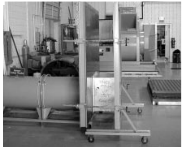
Damper Leakage Testing
