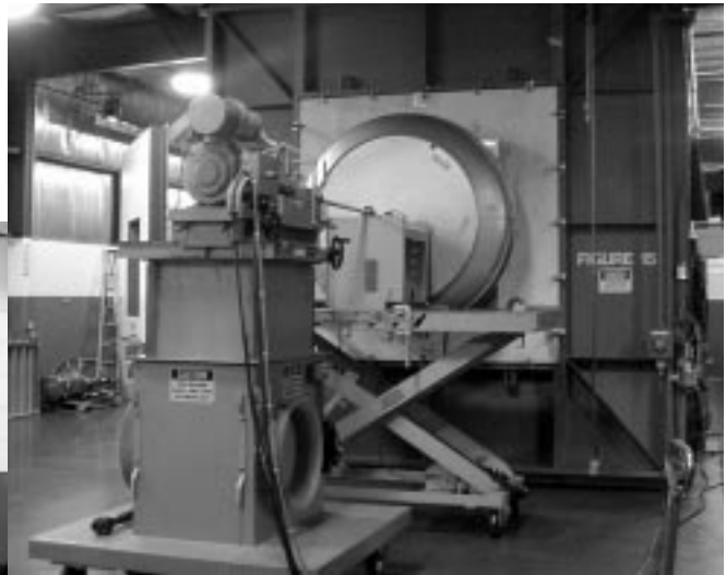
Air testing being conducted on a centrifugal roof fan
