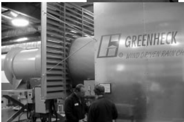
Damper being put through the test cycle on the wind driven rain tunnel
