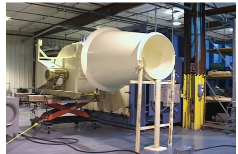
Photo B. Induced flow fan mounted on the outlet of a test chamber in Greenheck's AMCA-accredited air chamber.*
