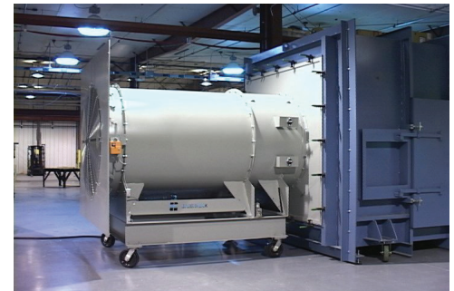
Photo C. Variable-supply and exhaust system used in an ANSI/AMCA Standard 210-99 test.
