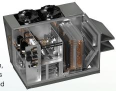
with a lead EC motor (standard feature). ASHPs are refrigeration systems that provide both cooling and heating. A reversing valve changes the direction of refrigerant flow, switching the system from cooling mode to heating mode. Supplemental and back-up heating options are available with the ASHP on the RV, RVE, and RVC.
