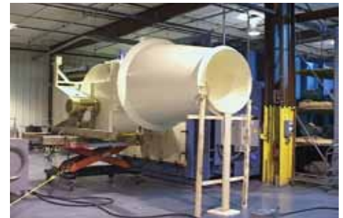
Photo B. High plume dilution blower mounted on the outlet of a test chamber in Greenheck's AMCA-accredited laboratory.
