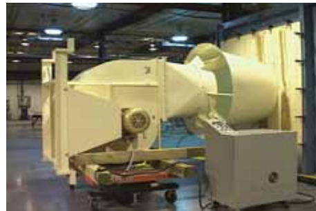
Photo A. High plume dilution blower mounted on the inlet of a test chamber in Greenheck's AMCA-accredited laboratory.
