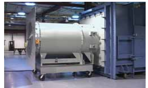
Photo C. Variable-supply and exhaust system used in an ANSI/AMCA Standard 210-99 test.
