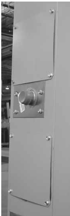
Distributor Access Panel
