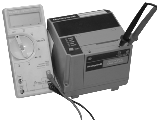
Figure 26. Flame Signal Check
