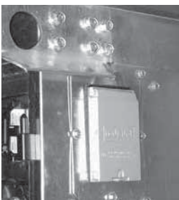
Manual High Voltage On/Off Switch with Lockout
