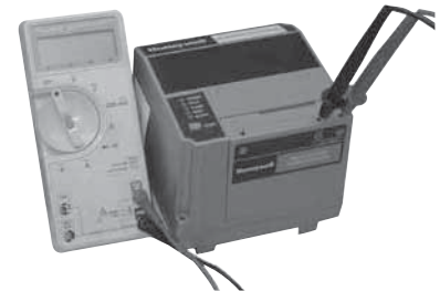
DC Voltmeter and Flame Amplifier
