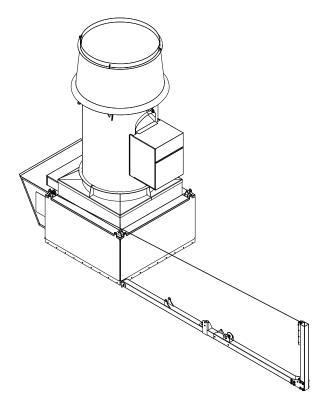
Step 5: Raise jib crane assembly by hand-lifting and using jib crane hand winch until fully erect.
