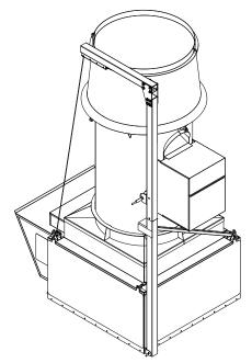
Step 8: Detach cable from hitch pin located at connection point 4 and remove hitch pin from connection point.
