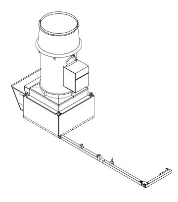
Step 4: Rotate jib crane boom straight up from the roof deck. Temporarily install one 1 x 4.75 inch hitch pin (E) into connection point 4 on the plenum. Lock hitch pin in place with cotter pin (G). Secure jib crane cable to now installed hitch pin located in plenum connection point 4 with crane hook.
