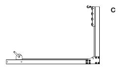
Insert boom over assembled post/pivot pad.
