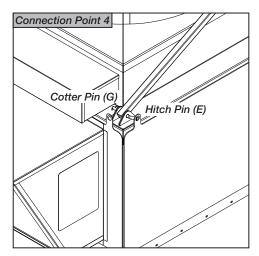
Jib crane assembly is now fully secured to the plenum. Refer to Vektor Installation, Operation and Maintenance Instruction for motor replacement procedure.
