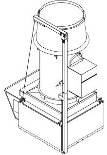
Step 7: At bracket connection point 3 and facing connection point 5, attach one support tube (F) at connection point 3 on jib crane using one 1 x 4.75 inch hitch pin (E). Lock hitch pin in place with cotter pin (G). Spread support tube out and attach the loose end to matching plenum connection point 5. Secure end with 1 x 4.75 inch hitch pin (E). Lock hitch pin in place with cotter pin (G).
