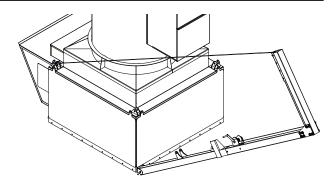
Step 6: Secure jib crane assembly to plenum at connection point 2 using one 1 x 6.75 inch hitch pin (D). Lock hitch pin in place with cotter pin (G). Make sure jib crane is firmly attached to plenum.
