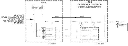
HL= HIGH LIMIT SENSOR P = PRIMARY TEMP SENSOR S1 = DAMPER POSITION INDICATION SWITCH, CLOSED WHEN DAMPER IS CLOSED. S2 - DAMPER POSITION INDICATION SWITCH, CLOSED WHEN DAMPER IS OPEN
