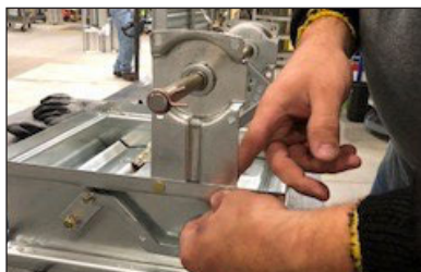
4. Nut and bolt jackshaft bracket to damper frame using pre-punched holes shown in the second photo. Repeat the steps for each section of damper.
