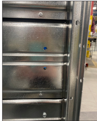
2. Determine the location where the blade jackshaft will be mounted (first or third blade). Note pre-punched holes in the jamb. Drill holes in blade according to Figure 1.
