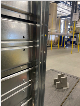
2. Determine the location where the blade jackshaft will be mounted (first or third blade). Note pre-punched holes in the jamb. Drill holes in blade according to Figure 1.
