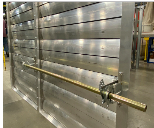
Figure 2: Drive Link Placement on Crankarm
