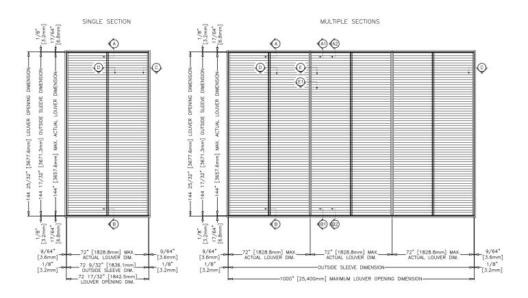
Minimum Rough Opening Size 12 in. W x 12 in. H Maximum Single Section Rough Opening Size 72.50 in. W x 144.50 in. H
