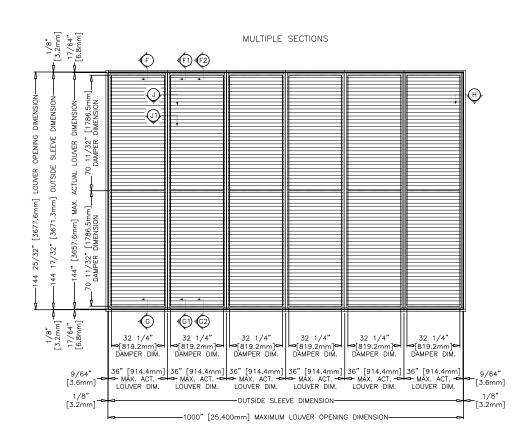
Minimum Rough Opening Size 12 in. W x 15.25 in. H Maximum Single Section Rough Opening Size 36.50 in. W x 144.50 in. H
