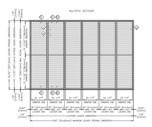
Minimum Rough Opening Size 12 in. W x 7 in. H Maximum Single Section Rough Opening Size 36.50 in. W x 144.50 in. H
