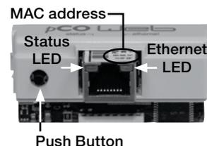
**Status LED:** Indicates the status of communication between the card and controller.
