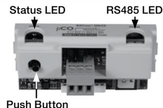
**Status LED:** Indicates the status of communication between the card and controller.
