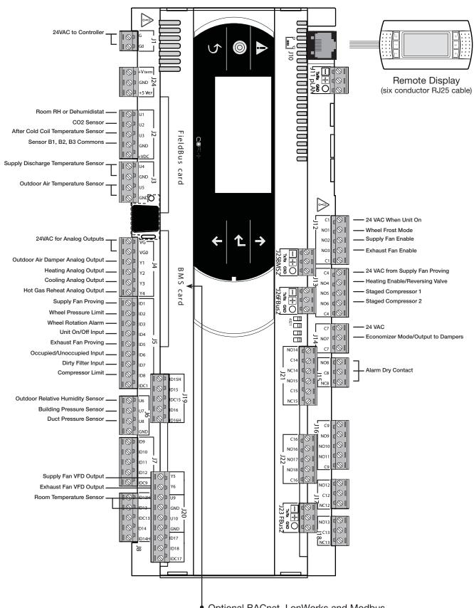
Optional BACnet, LonWorks and Modbus cards are located in BMS Card port
