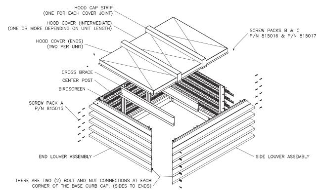
AFTER ASSEMBLY OF THE SIDES TO THE ENDS, ATTACH THE CROSS BRACE(S) TO THE SIDE CENTER POSTS PRIOR TO ATTACHING THE COVERS.
