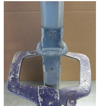
Figure 2: Clamping the blade open
