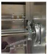
3. Loosen set screws on the actuator.
