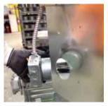
9. Loosen the bolts on the right side that holds the jackshaft bracket. Remove the jackshaft bracket on the left side. Loosen the bolts on the right side that holds the jackshaft bracket.
