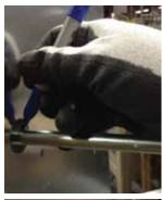
9. Remove retainer clip on the opposite end of the jackshaft.
