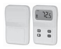
The room thermostat gives users the ability to view the room temperature and relative humidity (optional) and control the active room set points from the adjustable display. The room thermostat also has the ability to send the unit into temporary occupied mode. It is also provides the functionality to average up to 4 temperature readings through the microprocessor. The room thermostat is shipped loose with installation by others and is a Modbus connected device.
