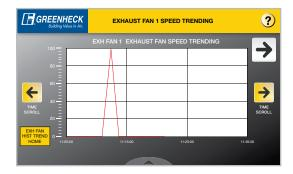
Trending provides additional information that shows history trending for exhaust fans, supply fans and temperature sensors. Scrolling forward or backward in time can be done using the orange colored arrow buttons.
