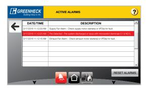
Alarms will show all current alarms. In the event of an alarm, the alarm page will automatically be displayed. The alarm description, date and time will be displayed for each current fault. If no faults exist, 'No Active Alarms' will be displayed. Once a fault is corrected, it will automatically be cleared.
