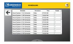
Allows the user to set up a scheduled time each hood system should turn on/off during the day. Can adjust the occurrence, time on and time off. In order for the scheduling to be used, the Enable check box must be selected.
