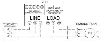
Each variable frequency drive must have the LINE and LOAD wiring in seperate conduit.
