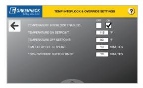
**Temperature Interlock Enabled:** User can enable or disable temperature interlock.
