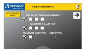
**Associated Temperature Sensors:** Link sensors to the hood by checking or unchecking the boxes.
