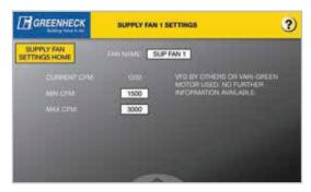
**Fan Name:** User can adjust the "nickname" of the fan to something such as "HOOD1 SUPPLY".
