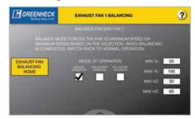
Balancing allows the user to easily balance the exhaust and supply fans.
