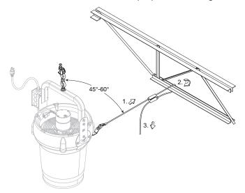
**NOTE:** Safety restraint cable will only feed through the Gripple connector in one direction (marked on the Gripple connector with an arrow). If necessary, the safety cable can be loosened by pressing the release
