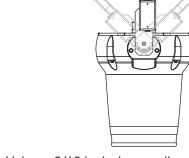
3. Using a 9/16 inch deep well socket, attach the eyebolt to the top of the fan handle.
