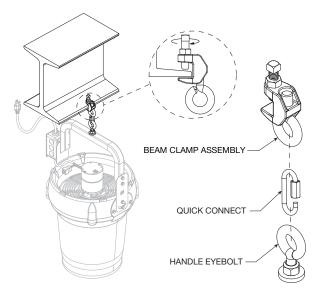
7. Wrap the loose end of the factory-installed safety restraint cable around the mounting structure so that the cable is installed 45° to 60° from vertical. Do not allow the cable to come in contact with any sharp edges.
