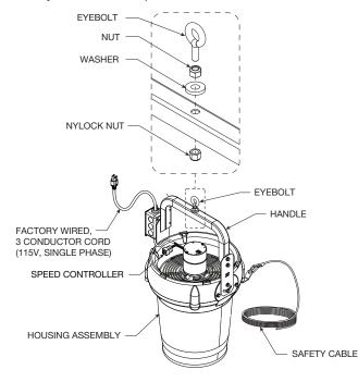
Attach the beam clamp assembly to the ceiling structure. Use the quick connect link to mount the handle eyebolt on the fan to the beam clamp assembly.
