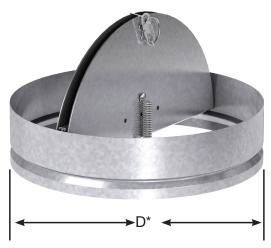
\*D dimension is actual O.D. of damper. If damper is to be installed inside duct work, order damper ¼ in. smaller than duct size.
