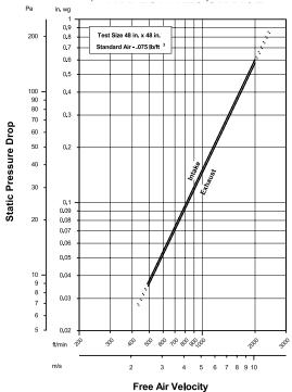
Model ESD-635HP resistance to airflow (pressure drop) varies depending on louver application (air intake or air exhaust). Free area velocities (shown) are higher than average velocity through the overall louver size. See louver selection information. (Test Figure 5.5-6.5)
