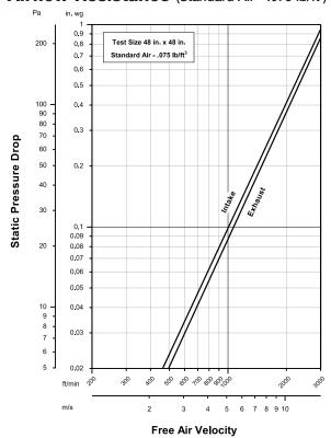
Model ESU-153 resistance to airflow (pressure drop) varies depending on louver application (air intake or air exhaust). Free area velocities (shown) are higher than average velocity through the overall louver size. See louver selection information.
