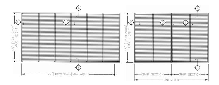
Minimum Single Section Size 13  $\frac{1}{2}$  in. W x 10 in. H (without flange) 13  $\frac{1}{2}$  in. W x 12 in. H (with flange)
