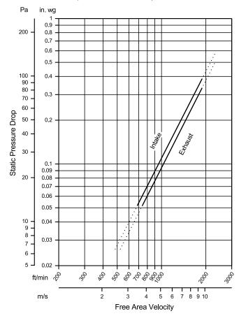
Model FAD-635 resistance to airflow (pressure drop) varies depending on louver application (air intake or air exhaust). Free area velocities (shown) are higher than average velocity through the overall louver size. See louver selection information. (Test Figure 5.5-6.5)
