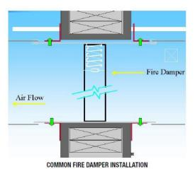
Example of a common fire damper installation:
