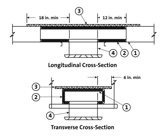
Item 1 – Steel Duct Item 2 – Glass Fiber Duct Lining Item 3 – Acoustical Lay-in Panel Item 4 – Ceramic Paper
