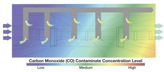
Ductless GJX System – Fresh supply air is pushed throughout the parking area towards the mechanical exhaust duct
