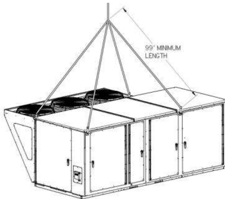
Figure 11 - Lifting Details of a 6-25 and 30 ton Energy Recovery Wheel or Power Return Unit
