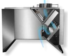
• By greatly reducing the need to heat a steady, one-way flow of water, the Grease Grabber H<sub>2</sub>O's recirculation method helps control utility costs. The recirculating pump also doubles as a purge pump to drain the water, eliminating the need for a gravity drain. A programmable timer allows for cleaning to be completed on a set schedule or by the push of a button.
