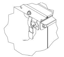
The latch kit will remain available as an option for tool-free hold closed of the fan.
