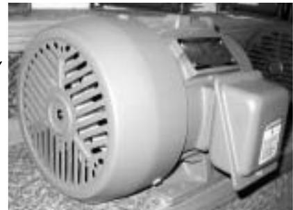
Totally Enclosed Fan Cooled Motor
