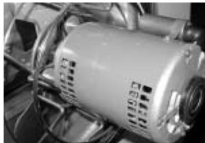
Thru bolt mounted motor
